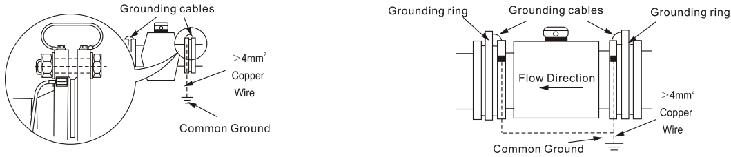
A. Metal pipe grounding
